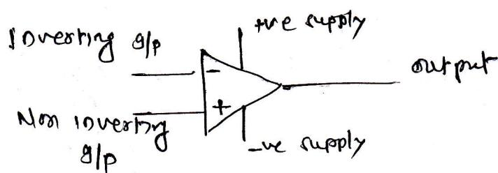
The terminal marked +ve is non inverting input and terminal marked -ve is inverting input of OPAMP. A signal applied at +ve terminal appears with same polarity and amplified at the output, while an input applied to -ve input terminals appear at the output with opposite polarity and with amplification as shown
