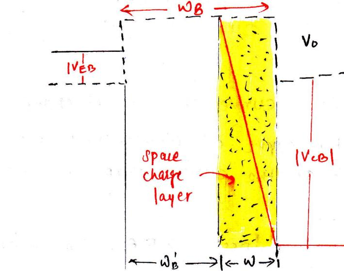
As per the explanation given the depletion layer penetrates more into base than collector. Hence collector depletion region is neglected. If the base width is  $W_B$ , then effective electrical base width is  $W_B' = W_B - w$  due to applied reverse bias at  $CB$  junction. This modulation of effective base width by collector voltage is known as Early effect. The decrease in  $W_B'$  with increase in reverse collector voltage has three consequences
