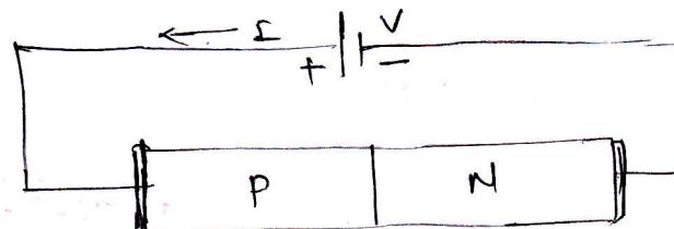
Hence the current can be considered only due to majority carrier drift and minority current (is only due to diffusion). The hole diffusion current in the N type material  $I_{pn}$  decreases exponentially as shown (with distance)
