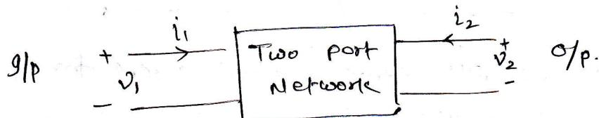
We can select two of four quantity as the independent variable and express the other two in terms of chosen independent variables. We can not choose independent parameter arbitrarily as in transformer \$v\_1\$ and \$v\_2\$ could not be taken as independent as their ratio is constant now if the current and voltage \$i\_1, v\_2\$ are independent and N/W is linear
