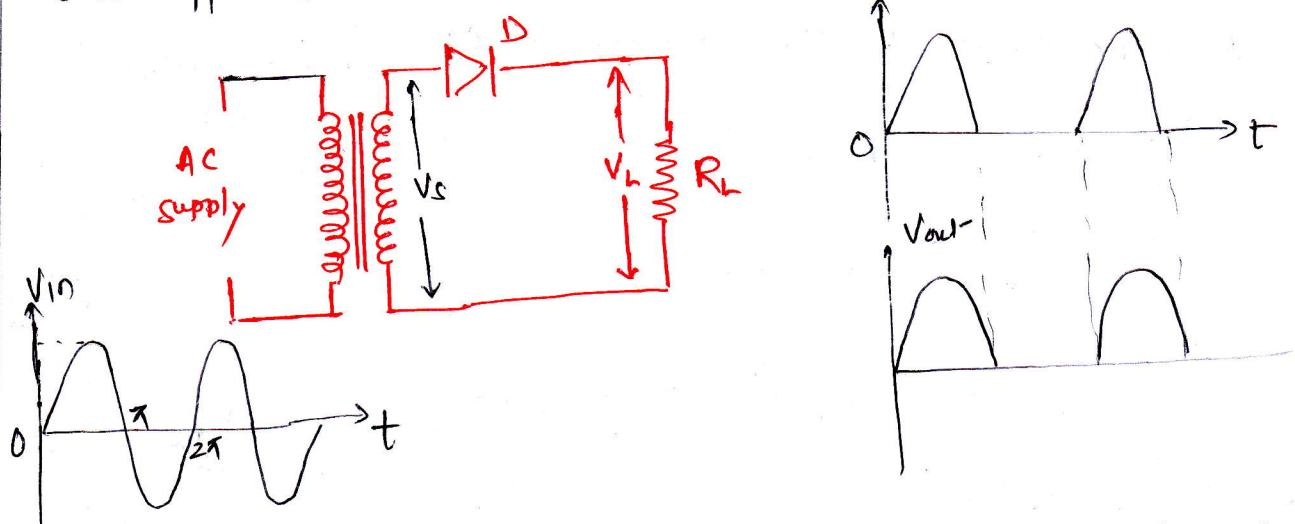
For +ve half cycle of o/p waveform diode P side is connected to +ve and N side to -ve and diode acts as forward biased and current flows from load  $R_L$  downwards and load voltage is +ve.
