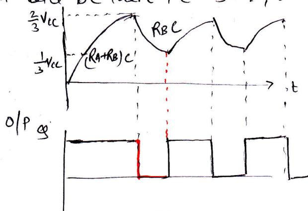
$$T_{HIGH} = 0.693 (R_A + R_B) C$$
