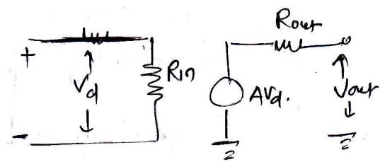
$$V_{out} = A_vd \cdot V_d = A(v_1 - v_2)$$
