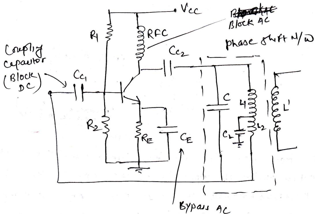
The output of the amplifier is given to LC tank circuit which is having one capacitor and two inductor. The voltage across inductor  $L_2$  forms feedback voltage.  $L_1$  or  $L_2$  can not be grounded directly i.e. why capacitor  $C_2$  is used. The feedback network provide  $180^\circ$  of phase shift to the amplified and inverted output of amplifier, total phase shift is now  $360^\circ$ . And above circuit oscillate at resonant freq of tank circuit given by
