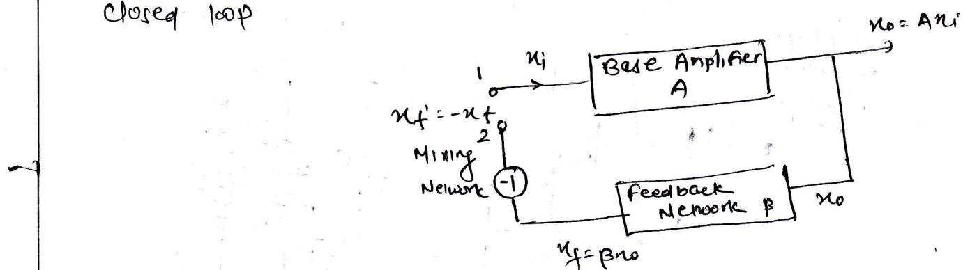
The base amplifier provides output signal  $n_o$  which is amplified version of input  $n_i$  as the input is  $n_i$ . The output of feedback network is  $n_f = \beta n_o = AB n_i$  and the o/p of mixing network is  $n_f' = -n_f = -AB n_i$ .
