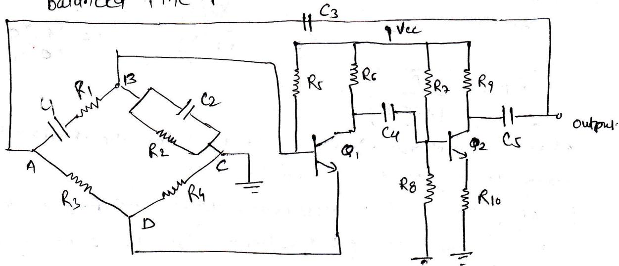
In the bridge circuit  $R_1$  in series with  $C_1$ ,  $R_3$ ,  $R_4$  and  $R_2$  in parallel with  $C_2$  form the four arm.
