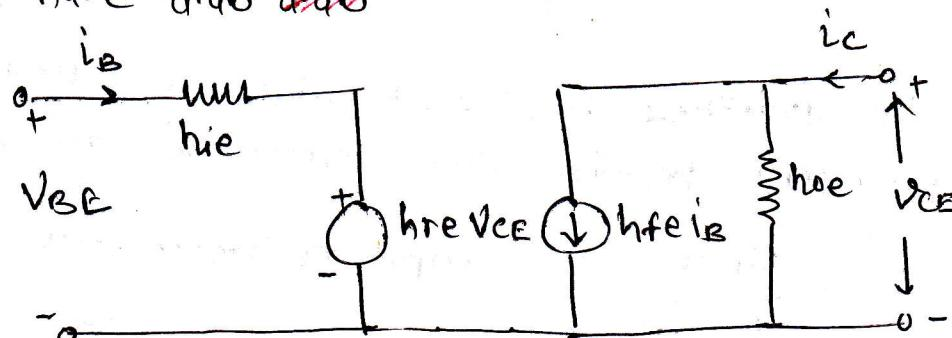
$$v_{BE} = h_{ie} i_B + h_{re} v_{CE}$$
