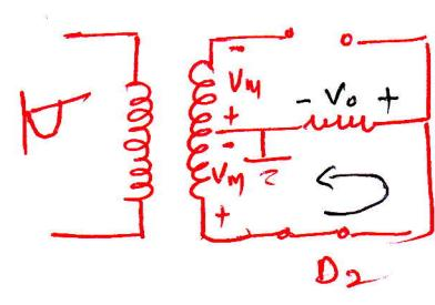
Full wave Rectifier circuit is shown in figure. For +ve half diode  $D_1$  is forward biased and acts as short circuit and current from load  $R_L$  is right to left. Similarly for -ve half of g/p waveform diode  $D_1$  is RB and  $D_2$  is FB and acts as short with  $D_2$  open as shown. direction of current from load  $R_L$  is again from right to left. So O/P current is alternating but O/P current ~~is~~ remains unidirectional. hence above circuit acts as rectifier.
